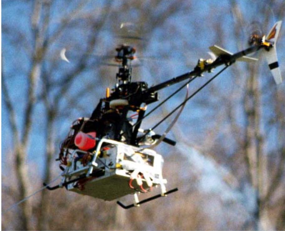
Figure 2-1: Instrumented X-Cell helicopter in flight
